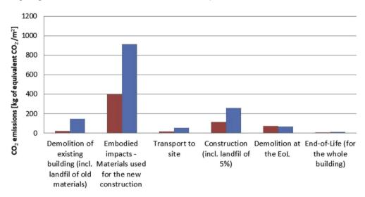
Fig. 3.  $CO_2$  emissions [kg of equivalent  $CO_2/m^2$ ] per phase, respectively for the *retrofit* project (red bars) and for the *rebuild* project (blue bars) (use phase is excluded). (For interpretation of the references to colour in this figure legend, the reader is referred to the Web version of this article.)
