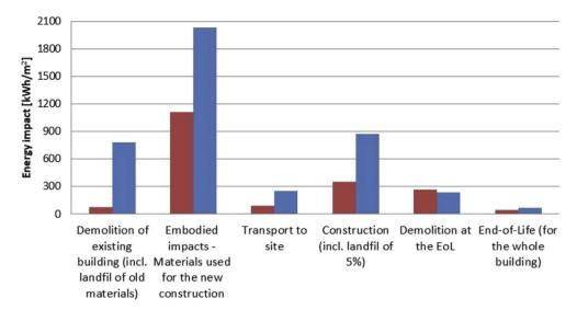
Fig. 2. Energy impact [kWh/m²] per phase, respectively for the *retrofit* project (red bars) and for the *rebuild* project (blue bars) (use phase is excluded). (For interpretation of the references to colour in this figure legend, the reader is referred to the Web version of this article.)
